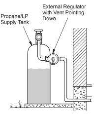
Figure 18 - External Regulator with Vent Pointing Down (Propane/LP Only)
